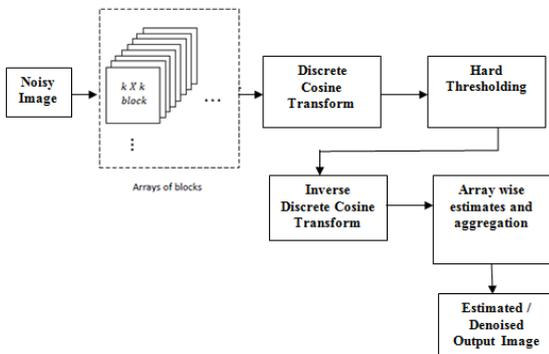
Figure 2: Block diagram of Block matching Discrete Cosine Transform (\*for third dimension processing Haar transform is used)
